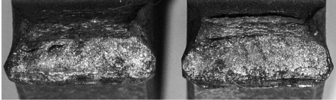
Fig. 10. Charpy specimen – notch type U 1
