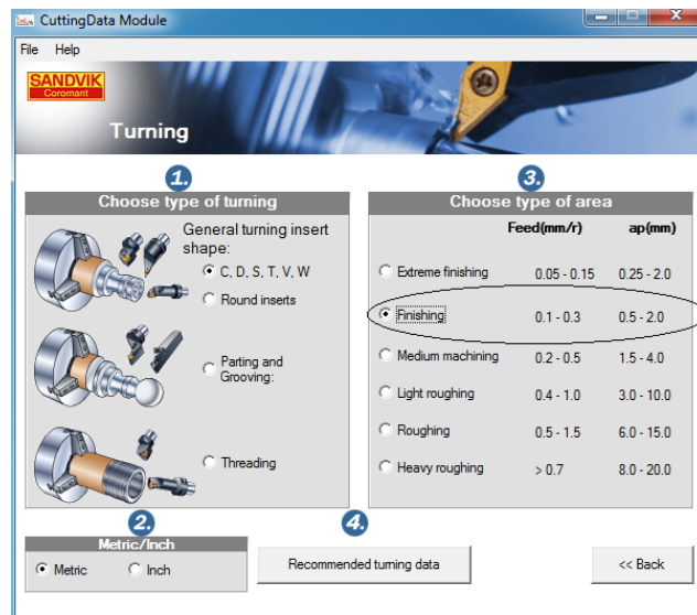
Fig. 5. Selection of feed work values ( f ) and cutting depth ( a_p ) [17]
