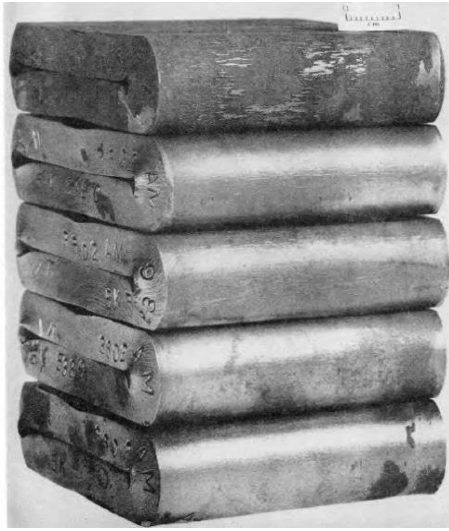
Fig. 5. Images of samples tested for flattening (from bottom to top), taken from tubes that operated 3000 hours at 482 °C, 538 °C, 593 °C, 649 °C, and 704 °C, respectively [17]
