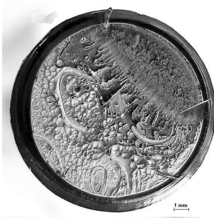
**Fig. 2.** Fracture surface of the OA1 sample
