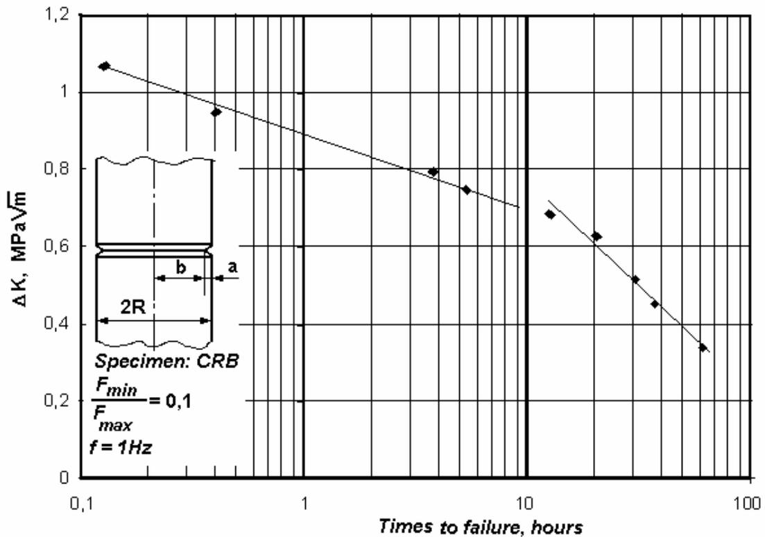
**Fig. 1.** Sample geometry and applied stress intensity factor vs. time to failure
