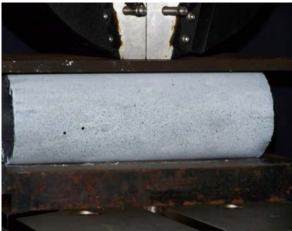
Fig. 1. Setting the pipe in the universal test machine
