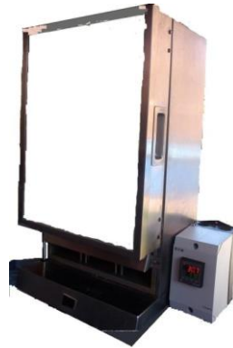
Fig. 2. Implementation of the temperature control system (the thermal enclosure and the Brainchild BTC-9100 controller)
