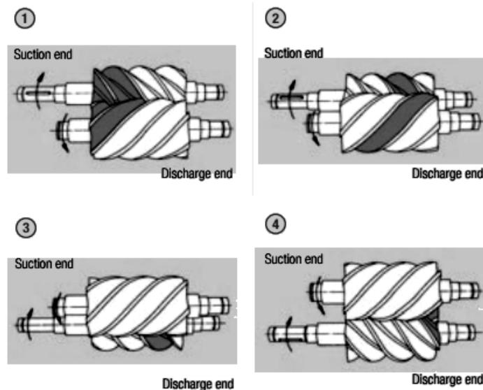
**Fig. 2.** Working phases of rotary screw compressor:
