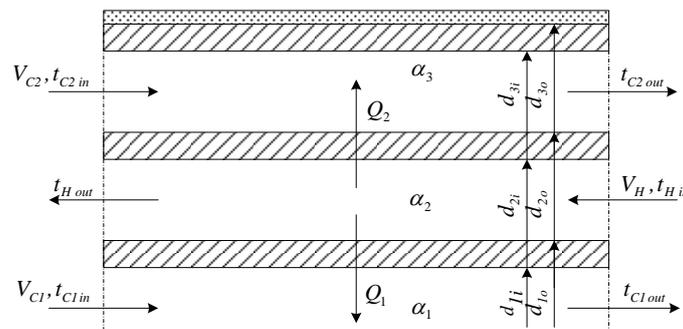
Fig. 1. The longitudinal section of the heat exchanger tubes
