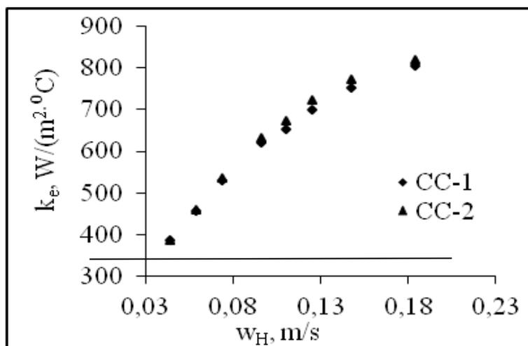
Fig. 3. The variation of  $k_e$  with the linear average velocity of hot water
