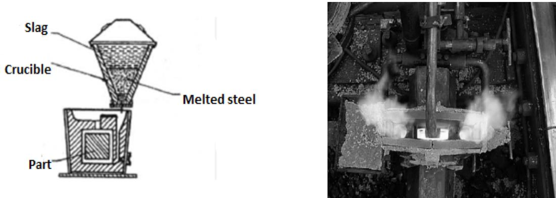
**Fig. 1.** Thermite welding [2]
