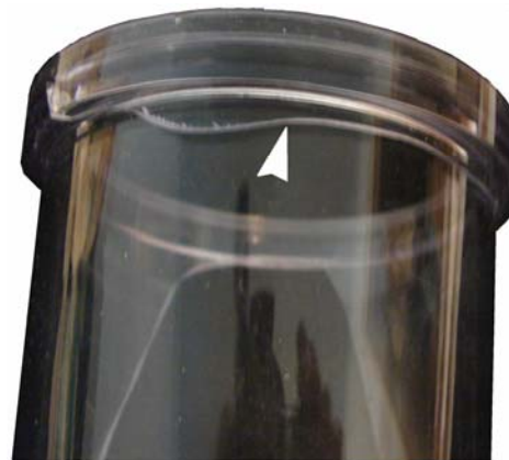
Fig. 2 The filter body cracked
