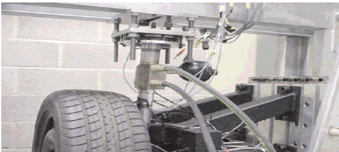
Fig. 2. Test stand for testing the quarter-car type suspension (1/4M)
