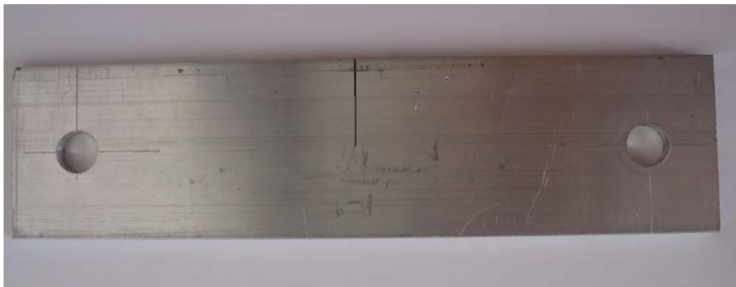
Fig. 2. The AL6060T6 non-standardized test specimen
