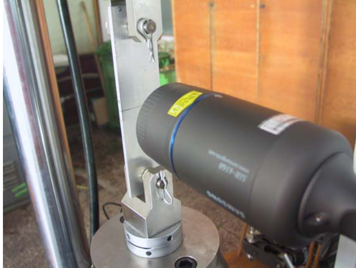
Fig. 4. The compact size allows easy placement of the video camera on the side of the specimen
