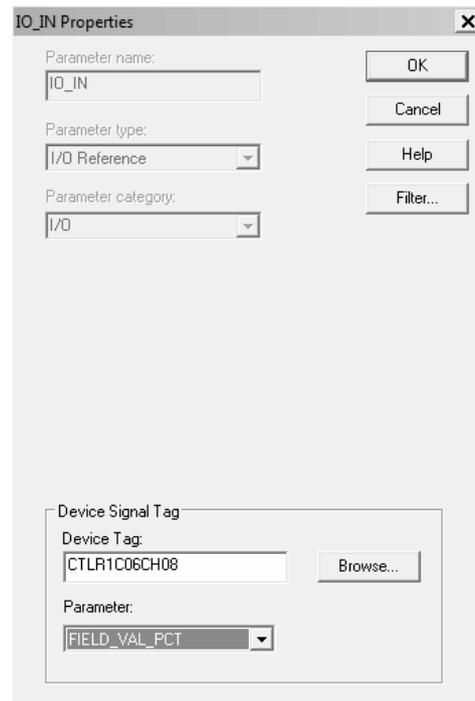
**Fig. 6.** The assignment of AI block with the analog input channel.
