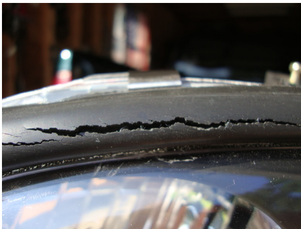
Fig. 7. Crack in a tire [6]
