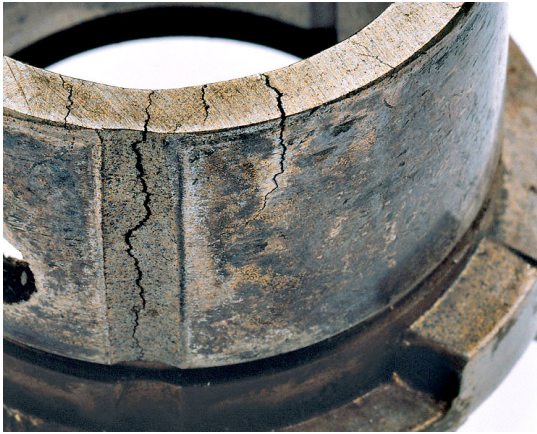
Fig. 5. Cracks in a piece of composite material [4]
