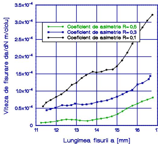
Fig. 3. Cracking rate versus crack's length
