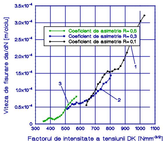
Fig. 5. Cracking rate in function SIF  $\Delta K$
