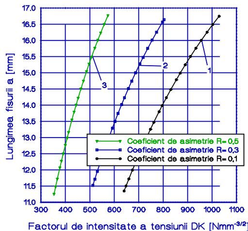
Fig. 4. Crack's length versus SIF  $\Delta K$
