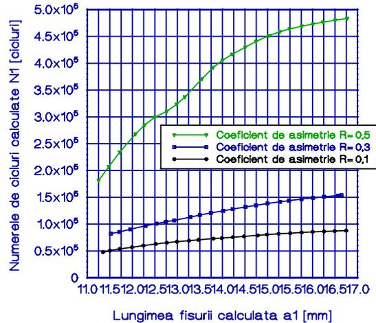
Fig. 2. Durability variation versus crack's length
