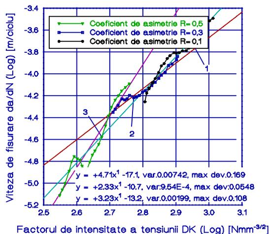
Fig. 6. Crack growth rate versus SIF  $\Delta K$  ( logarithmic co-ordinates )
