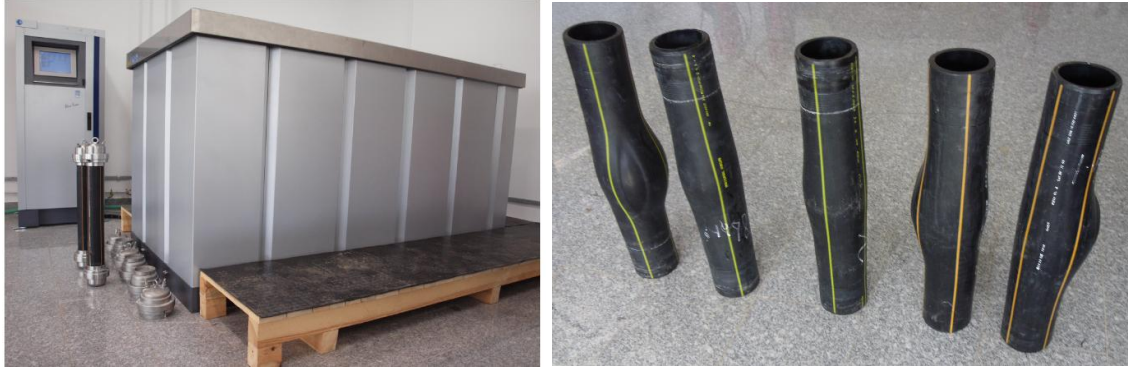
Fig. 6. Installation for mechanical testing of polyethylene pipes
