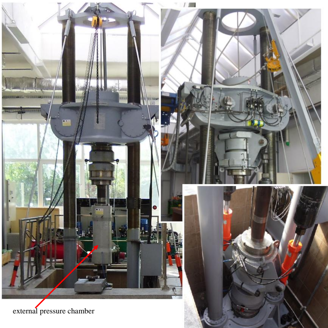
Fig. 2. Installation for testing OCTG under combined loadings
