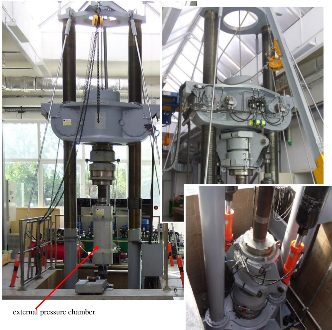
Fig. 2. Installation for testing OCTG under combined loadings
