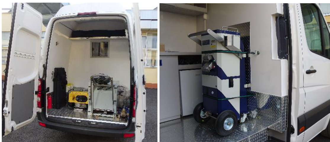
Fig. 11. Mobile laboratory for non-destructive testing of OCTG
