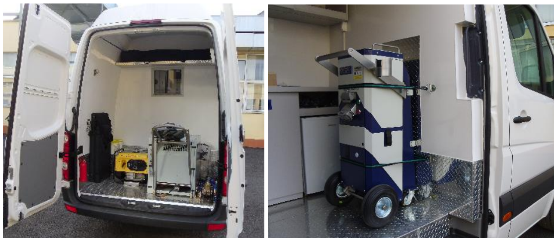
Fig. 11. Mobile laboratory for non-destructive testing of OCTG
