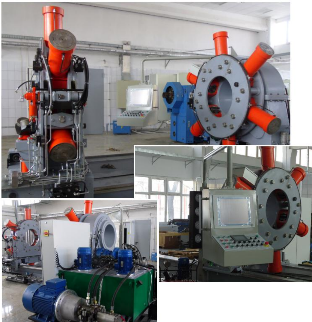
Fig. 5. Make up / break out testing machine
