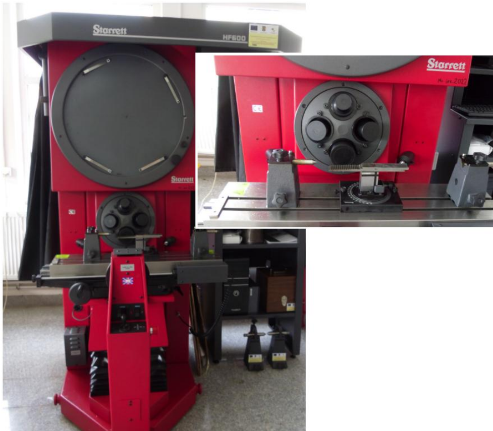
Fig. 7. Microscope for threads
