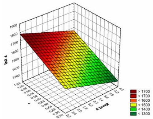
(b) Variation graph of the force at which the cylinder moves, function of the depth (length) of the cylinder and the defect area
