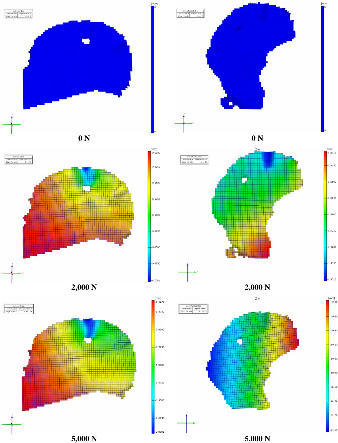
**Fig. 10** Displacement on vertical direction (Oy) at the loading of the osteochondral cylinder that does not reach the base of the receiving tunnel
