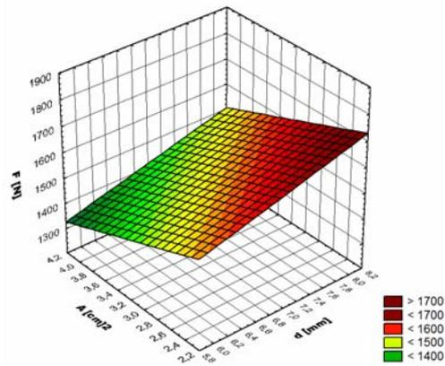
(a) Variation graph of the force at which the cylinder moves, function of the cylinder diameter and the defect area
