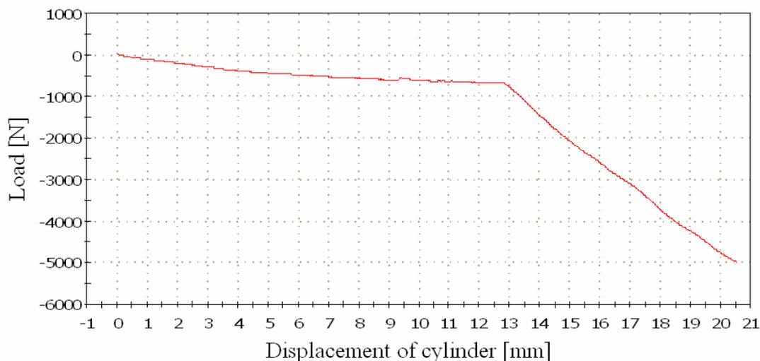
**Fig. 5** The variation of force during compressing the femur with a transplanted osteochondral defect ( $D_{\text{cyl}} = 8 \text{ mm}$ ,  $A = 2,5 \text{ cm}^2$ ) with up to 5,000 N
