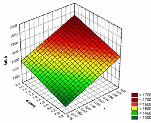
(c) Variation graph of the force at which the cylinder moves, function of the cylinder diameter and the ratio between the tunnel depth and the cylinder length
