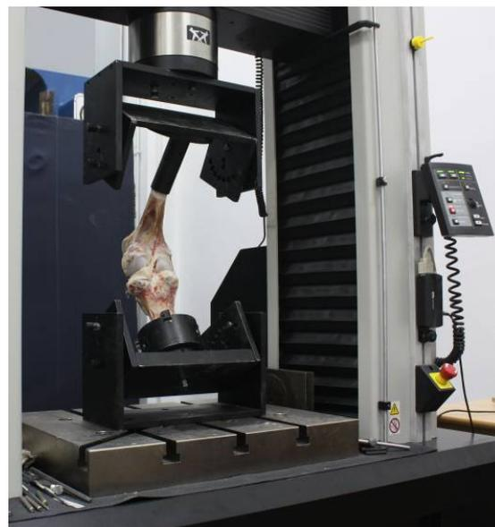
**Fig. 4** Fastening of the bovine knee in the Instron machine
