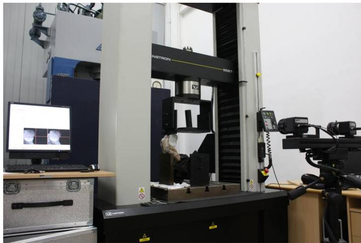
**Fig. 9** Fastening of the bovine knee in the Instron 5587 machine using the experimental device and positioning of the Aramis 2M system for acquiring the experimental data
