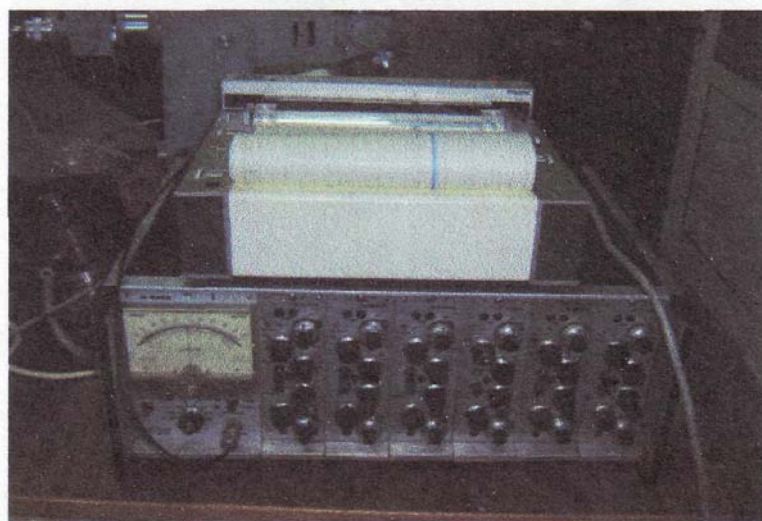
Fig. 1. Tensiometric bridge and graphs register
