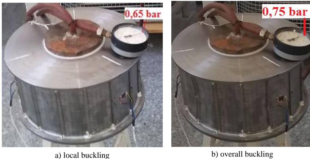
Fig. 3. Local and overall buckling shapes for stiffened shell under uniform external pressure
