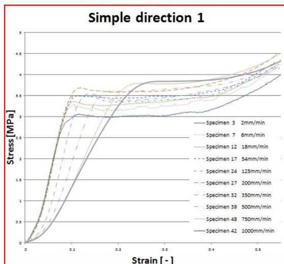
Fig. 2. Compression response of the simple foam on direction 1
