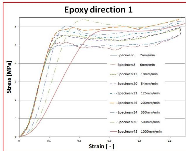
Fig. 3. Influence of impregnation with epoxy resin on direction 1
