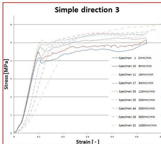
Fig. 1. Compression response of the simple foam on direction 3
