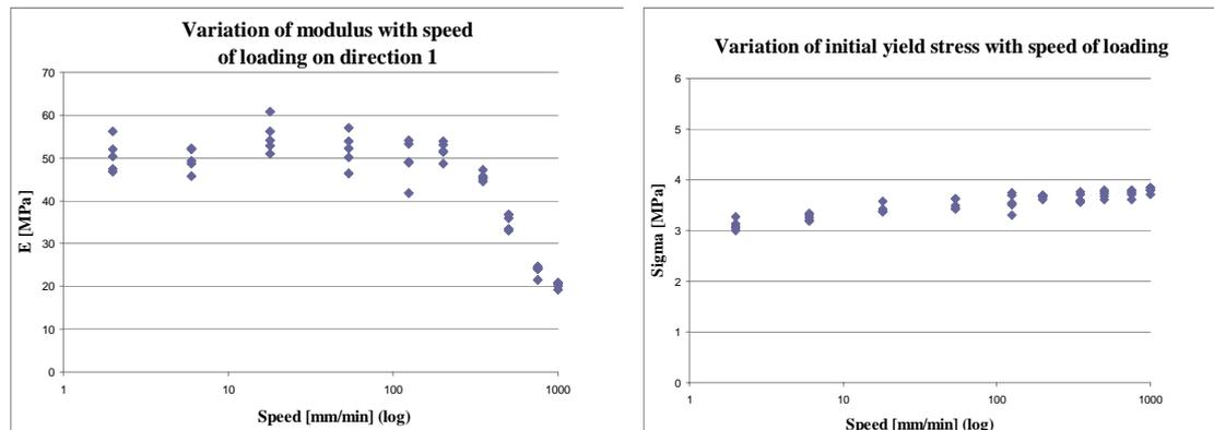
**Fig. 7.** Variation of the modulus and initial yield stress with the speed of loading on direction 1
