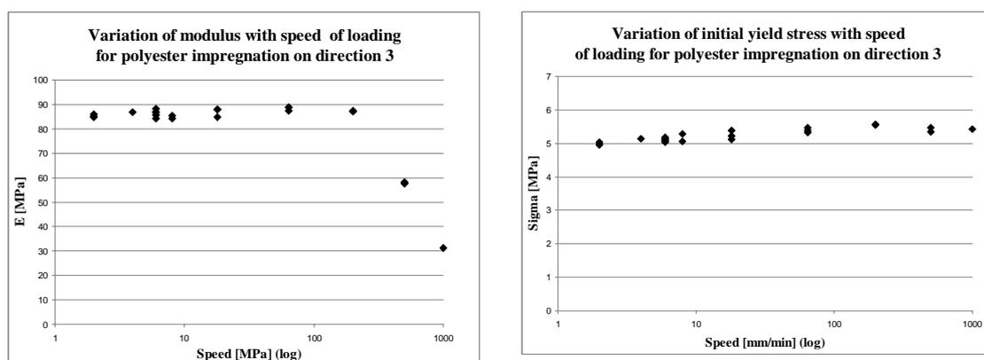
Fig. 9. Variation of the modulus and initial yield stress with the speed of loading on direction 3
