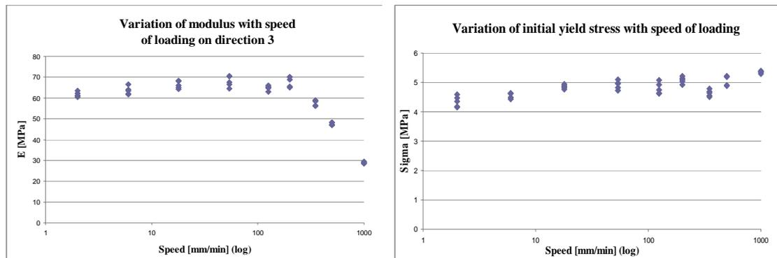
**Fig. 6.** Variation of the modulus and initial yield stress with the speed of loading on direction 3
