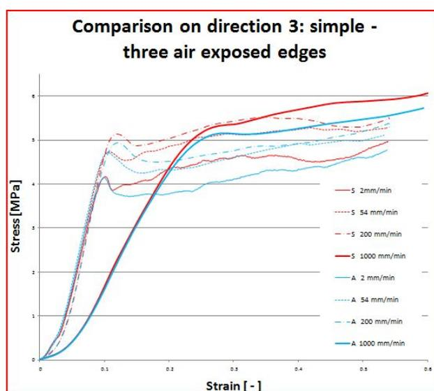
Fig. 5. Comparison of simple to air exposed foam on direction 3
