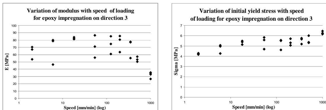
Fig. 8. Variation of the modulus and initial yield stress with the speed of loading on direction 3
