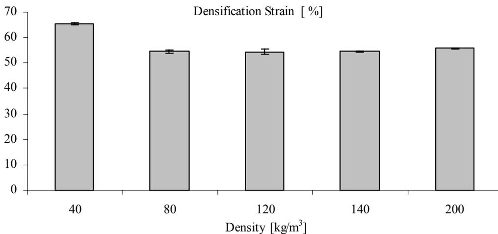
**Fig. 8.** Densification strain versus density
