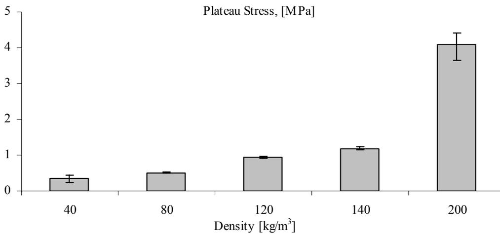
**Fig. 6.** Plateau stress versus density
