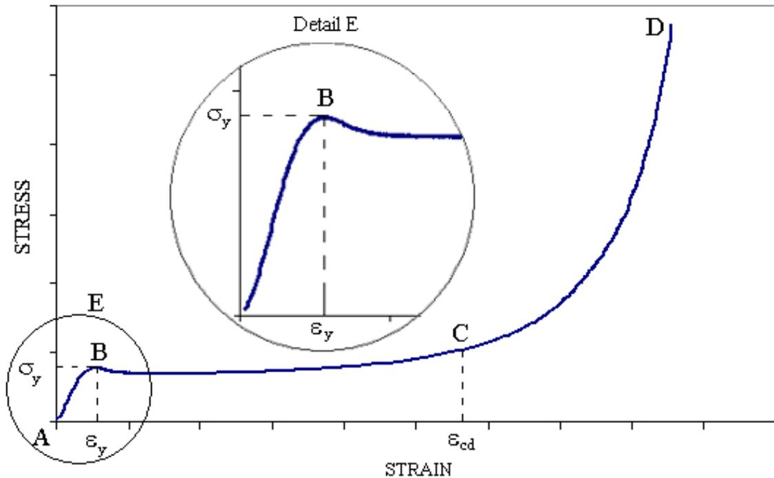
Fig.1. Stress-strain curve typical for rigid polyurethane foam
