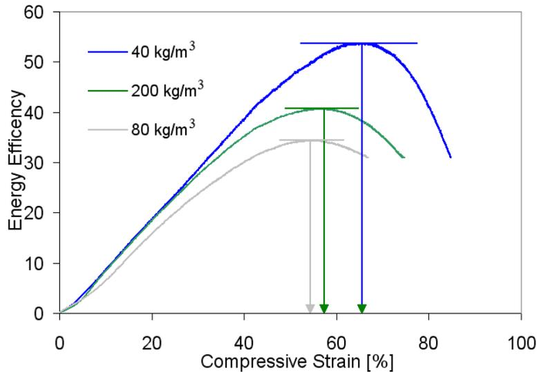
**Fig. 7.** Energy efficiency-Strain curves of three densities (40, 80 and 200 kg/m<sup>3</sup>)
