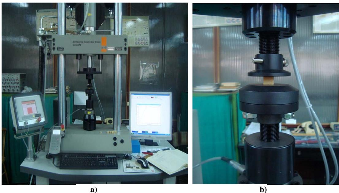
**Fig.3.** Walter Bay 10 kN testing machine
