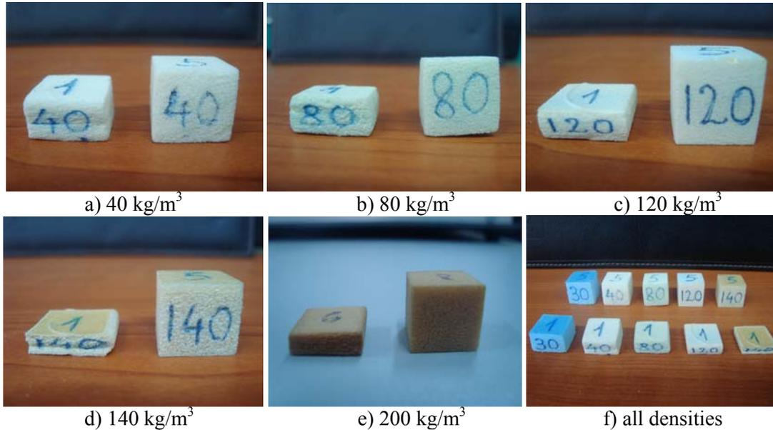
**Fig.2.** Compression specimens
