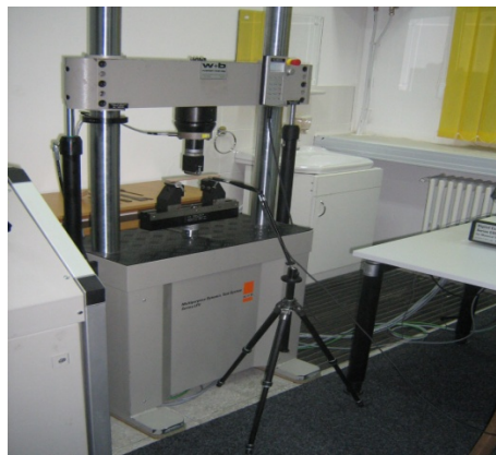
Fig.6. Charpy bending tests
