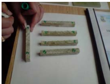
Fig.4. Specimens reinforced with nylon fiber
