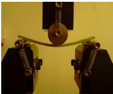
Fig.7. Specimens reinforced with nylon fiber
