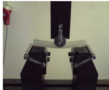
Fig.8. Specimens reinforced with nylon
