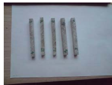
Fig.5. Specimens reinforced with nylon
