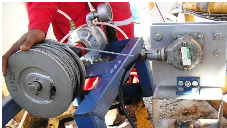
Fig. 4. Detail on pneumatic spooler from a geograph transducer[9].
