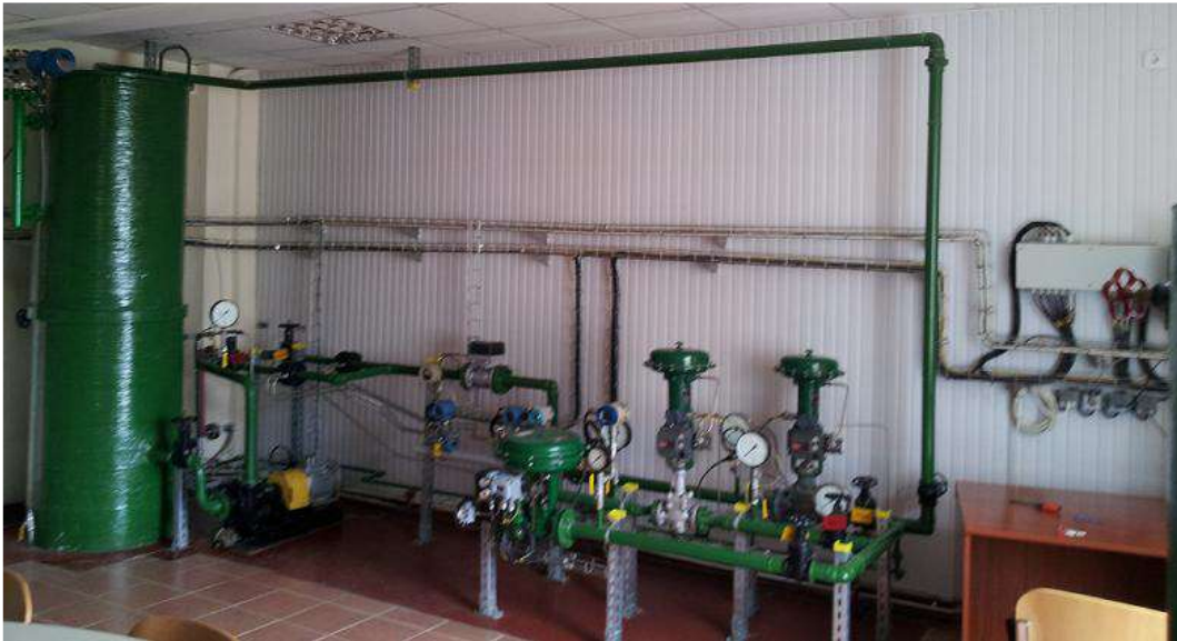
Fig. 1. The laboratory plant for tank level control.
