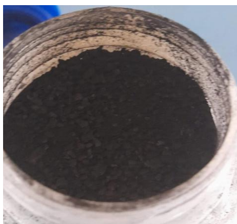
Figure 5. Completely carbonized corncob char.
