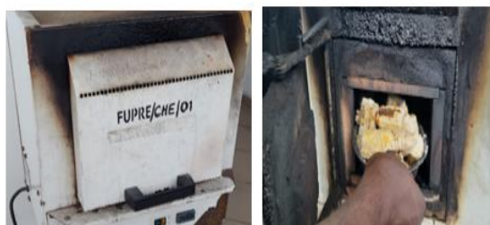
Figure 4. Carbonization of corncob in a Vecstar Furnace
