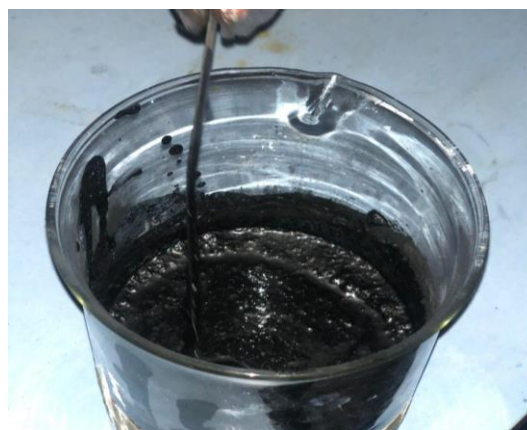
Figure 6. Activation of Corncob Char
