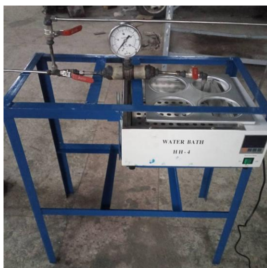
Figure 9. Experimental setup for evaluation of methane adsorption capacity
