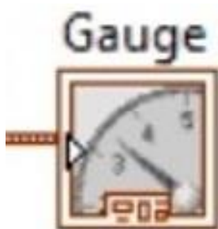
Figure 16. Function block for displaying the real-time displacement of the indicating needle in gauge-style
