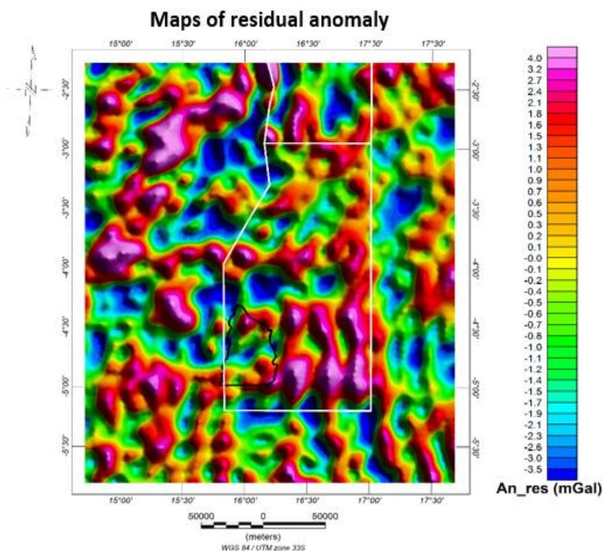
Figure 4. Residual anomalies map developed using Surfer software
