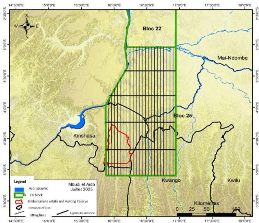
Figure 7. Gravity and magnetic survey planning developed using Surfer software
