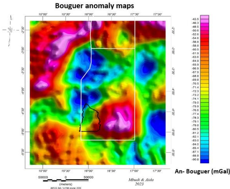
Figure 2. Bouguer anomaly map developed using surfer software
