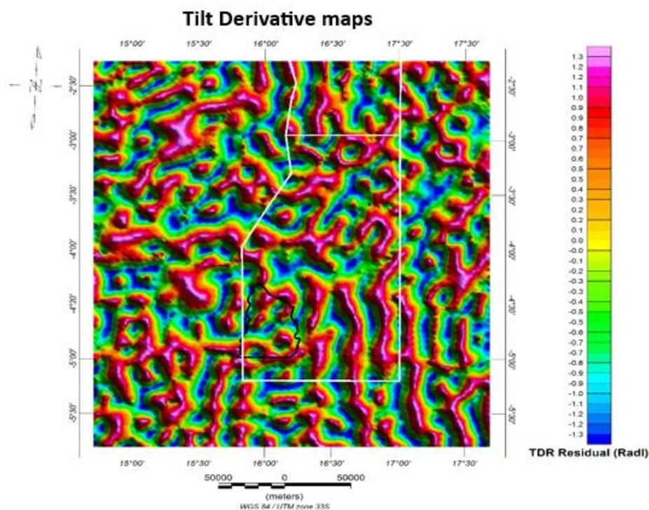
Figure 5. Tilt Derivative for residual anomalies developed using Surfer software
