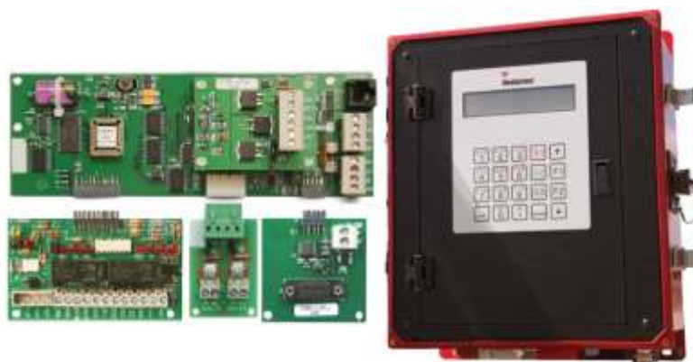
Figure 4. Weatherford gas well monitoring system [9].
