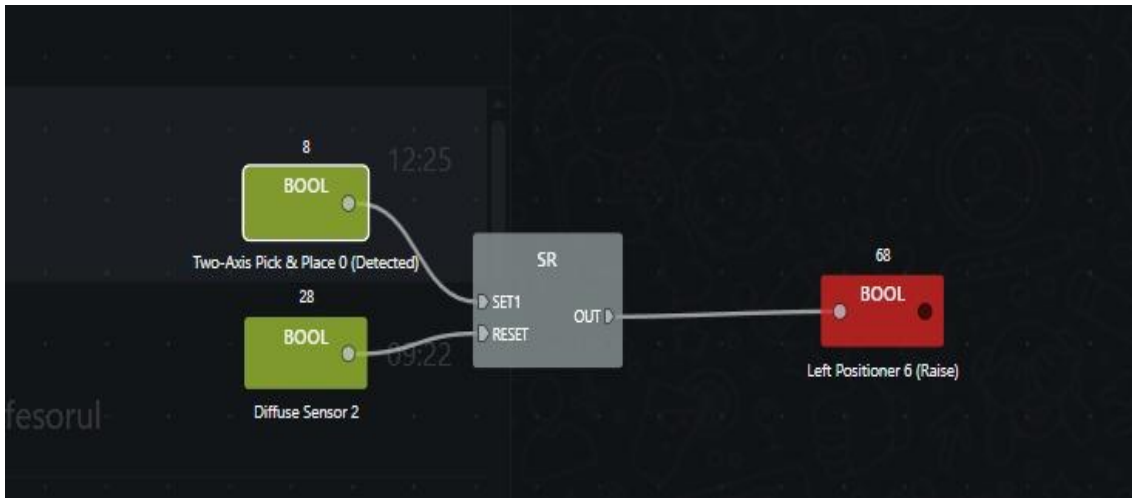
Figure 13. Barrier I raising / lowering conditions (Factory I/O)
