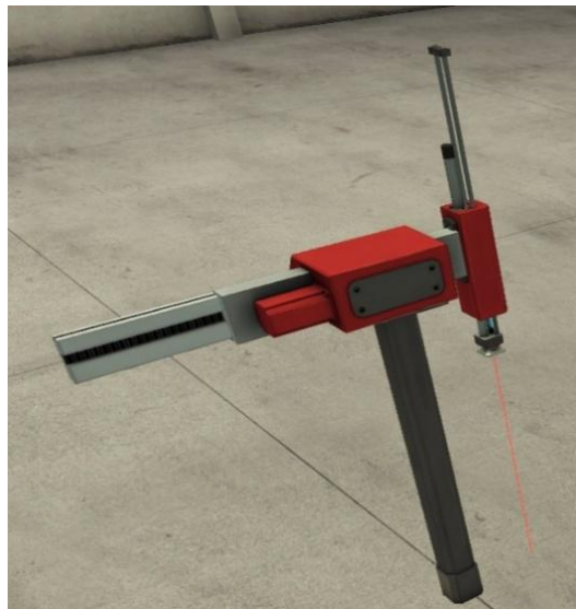
Figure 5. Robotic arm for assembly, with 2-axis movement (Factory I/O)
