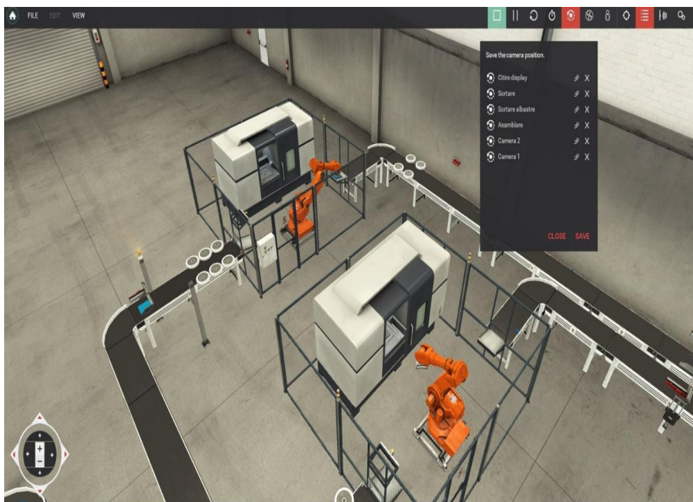
Figure 16. Screenshot of the two processing machines working in parallel (Factory I/O)
