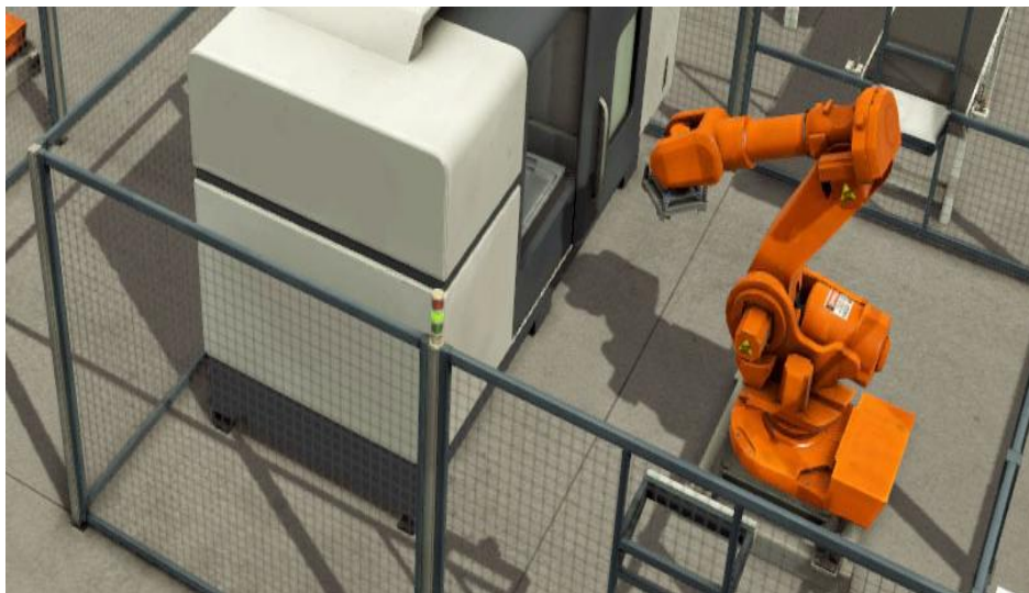
Figure 4. Part reception / processing / ejection subsystem (Machining center) (Factory I/O)
