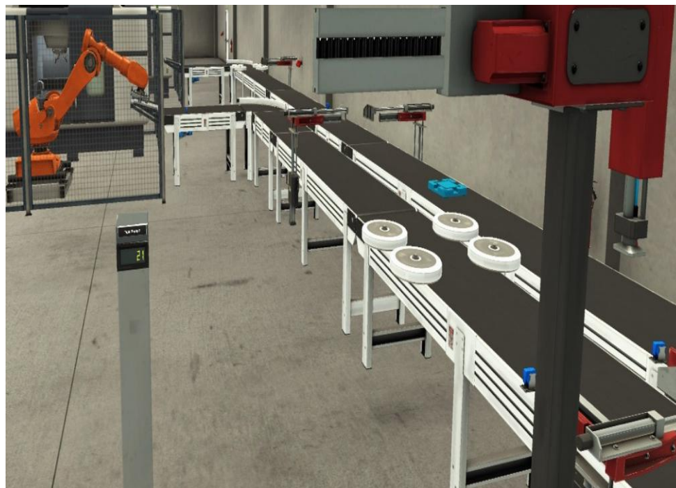
Figure 18. Screenshot of the assembly machine and the counter of correctly assembled parts (Factory I/O)
